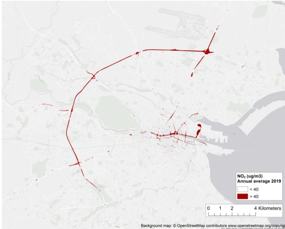
Figure F.20 – Coupled system modelled exceedances of annual average NO 2 AQSR limit (40 µg/m 3 ) in Dublin for 2019.
