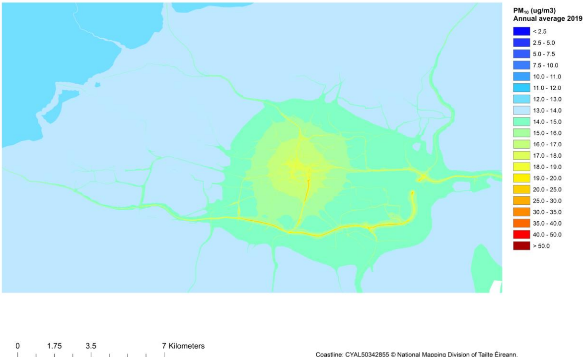
Figure F.14 – Coupled system annual average PM 10 city pollution map for 2019 of Cork; transition to exceedance of AQSR limit (40 μg/m 3 ) shown in bright red .
