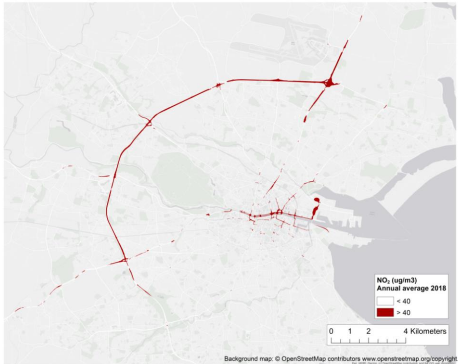
Figure F.16 – Coupled system modelled exceedances of annual average NO 2 AQSR limit (40 µg/m 3 ) in Dublin for 2018.
