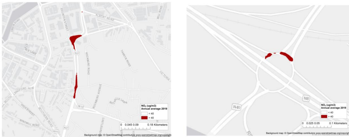
Figure F.23 – Coupled system modelled exceedances of annual average NO 2 AQSR limit (40 µg/m 3 ) in central Cork locations for 2019.
