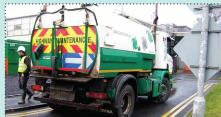
03 Use a road sweeper with a recirculating water system.
